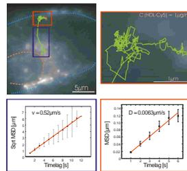
Uptake of HDL-Cy5 in a IdIA7-SRBI cell was followed as an intensity laps. The uptake of an individual HDL particle (upper right figure) shows trapping at the plasma membrane (red box) and directed transport (blue box) to the perinuclear region inside the cell. Analysis of such trajectories revealed an average diffusion constant of  $D = 0.004µm²/s$  and an average velocity of  $v = 0.43µm/s$
